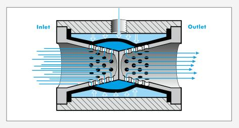
Unlike the design of conventional control valves, the sleeve and perforated cone assembly of the SF10V can maintain consistent pressure while letting process fluids from the separator pass through the valve.
